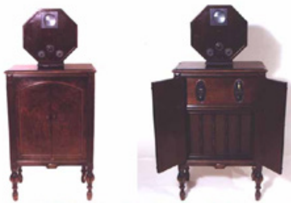
1928 G.E. Scanning Disk Television Set (closed-open)
